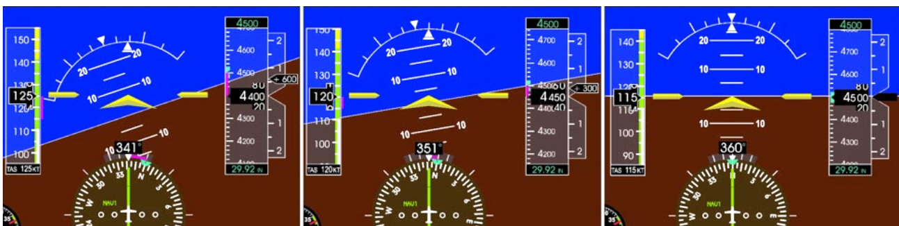
Figure 24. The magenta trend lines can be used to help you determine when to begin level off or roll out.
