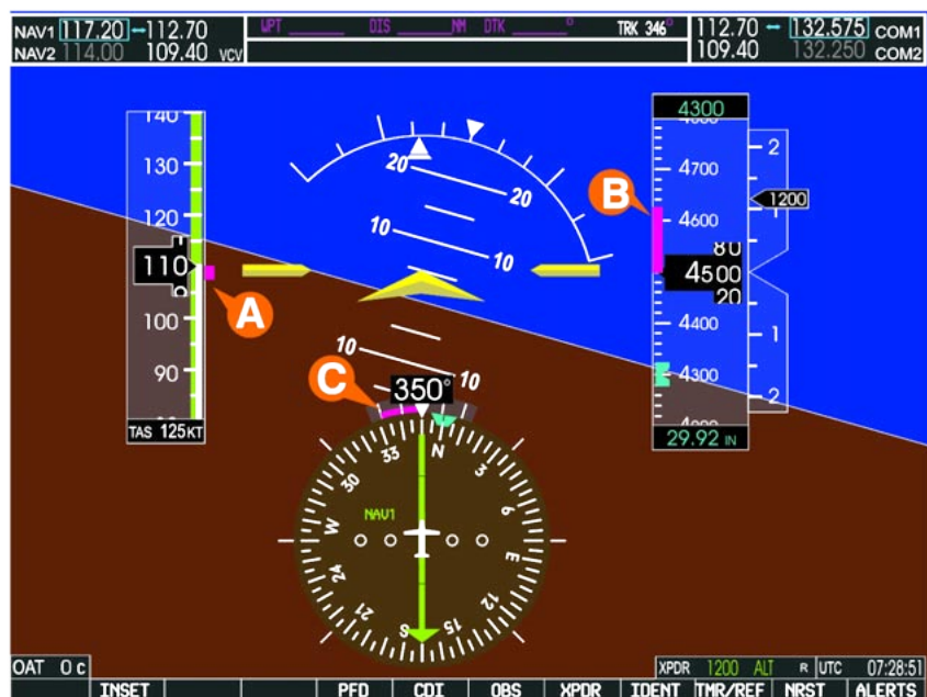
Figure 14. The magenta trend (vector) lines on a PFD (climbing) extend to where the airplane will be six seconds in the future.
