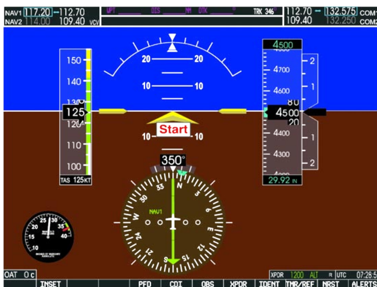
Figure 18. The instrument scan always begins with the attitude indicator.
