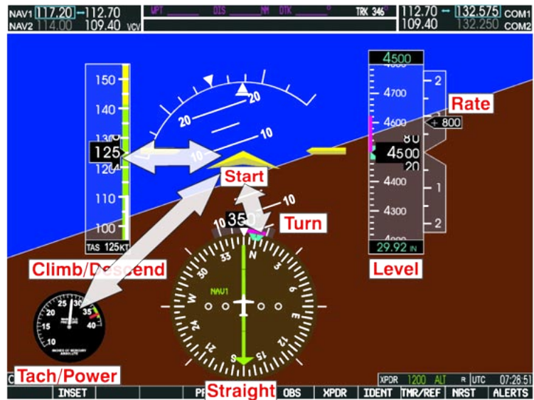
Figure 23. The scan above shows the primary instruments for a climbing right turn at 125 knots.
