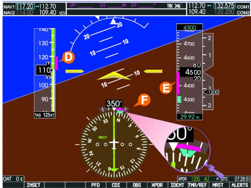
Figure 15. The magenta trend (vector) lines on a PFD (descending) extend to where the airplane will be six seconds in the future.
