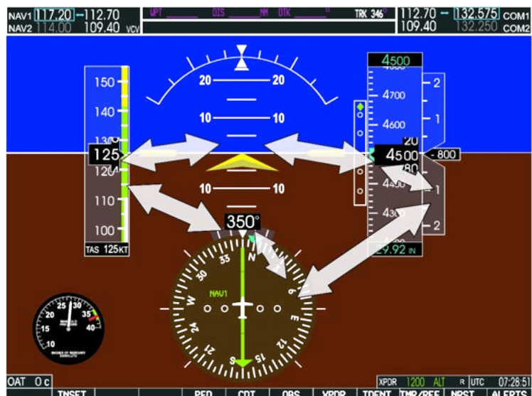
Figure 26. Scanning the 6-Pack cluster of instruments can be done to the right or to the left in a circular pattern.
