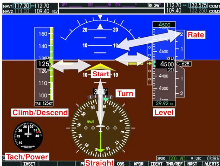
Figure 25. The scan above shows the primary instruments for an ILS approach (constant airspeed/rate descent).
