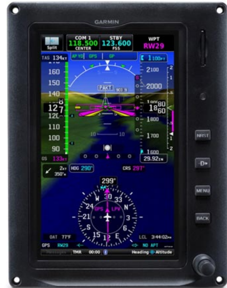
Garmin's portable GPS units (and other manufacturers, too) provide pitch and turn information in the cockpit.
