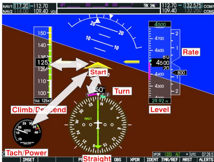
Figure 22. The scan above shows the primary instruments for a descending left turn at 125 knots.
